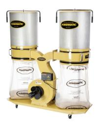
The PM-1900TX Dust Collector features the exclusive TurboCone&trade, which improves chip separation to prevent clogging of the filter, and increases packing efficiency of the collector bag. The canister filter offers superior filtering surface area over standard bags, and captures 98% of 2-micron particles. The all-metal duct improves
